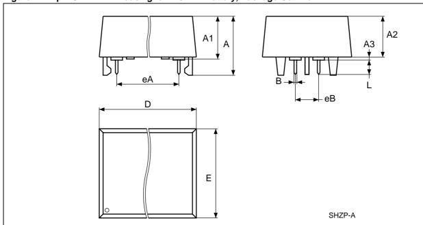
Figure 11. 4-pin SNAPHAT Housing for 120mAh Battery, Package Outline
