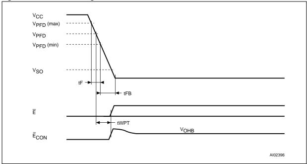
Figure 7. Power Up Timing
